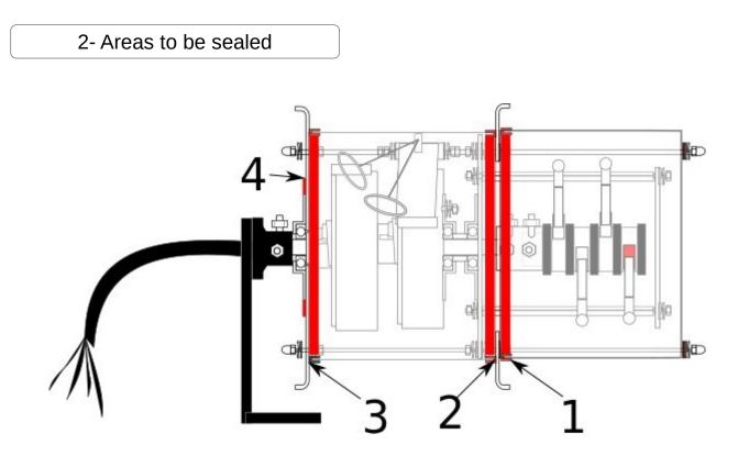
1- Following the rubber that seals the pot with the reel's wing 2 & 3- Following the rubber that seals the wings of the reel to the central body.
